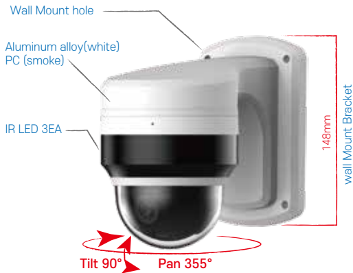
▶ Wall Mount Type installation Dimensions
